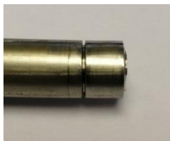
Figure 5 - Groove cut in tube for Push Fittings
